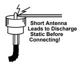
Important Warning: Never applying an external voltage to the Antenna jack -- it could damage sensitive detector diodes. Also, always discharge the coax connector to bleed off static before attaching ungrounded arrays.
