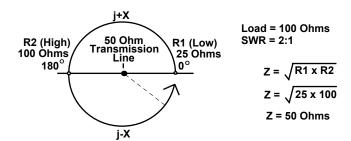
Viewed on a Smith Chart, the transformed load impedance ( $R \pm jX$ ) literally traces a circle around the characteristic impedance of the transmission line with each 360-degrees rotation. The greater the mismatch, the larger the diameter of the circle. We can use this behavior in two different ways to determine the impedance of an unknown transmission line.
